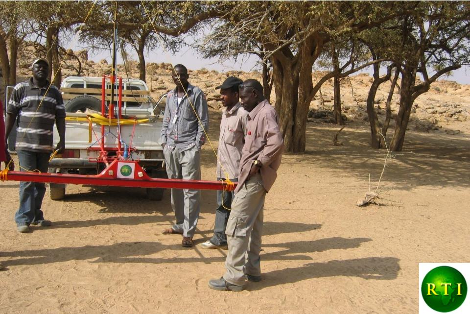
Record completed by a 400 Mhz GPR antenna to check the validity of the WATEX© image with an accuracy: 50 cm
